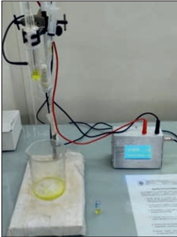
Fig. 4: Dose measurement setup of Ceric Cerous electrochemical cell and potentiometric measurement of dose using developed improved millivolt meter.
