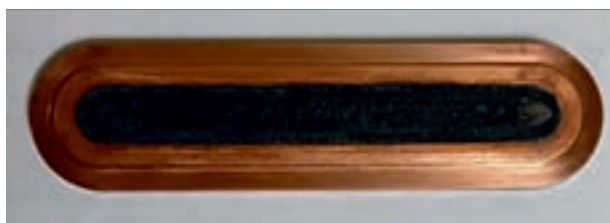
Fig. 1. Electroplated enriched Tl-203 target
