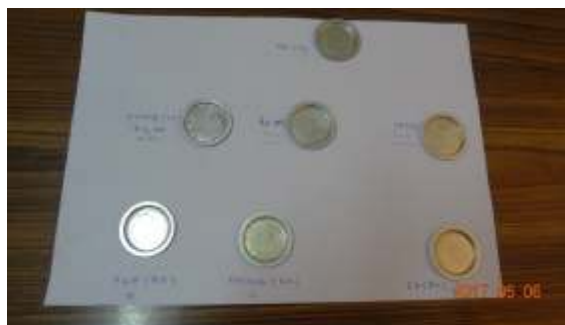
Fig. 1: Planchets with different polymers, EP- epoxy polymer, PMMA- Polymethylmethacrylate, PVP- Polyvinyl pyrrolidone
