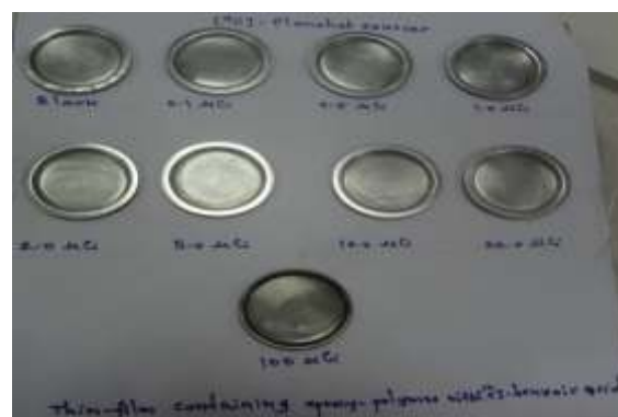
Fig. 2: [ 14 C]-Planchets prepared with the epoxy polymer
