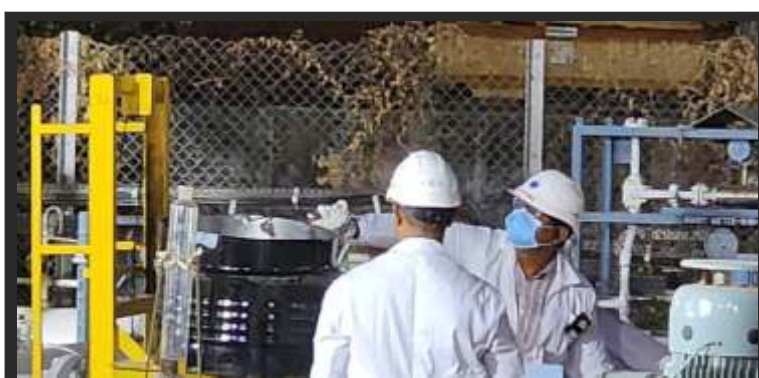
Fig. 3: BRIT team performing radiotracer injection at MDT
