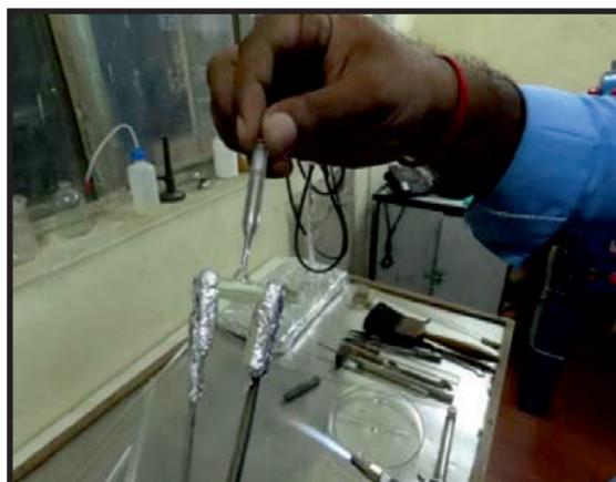
Fig. 8: Glass blowing set-up of Spl sources
