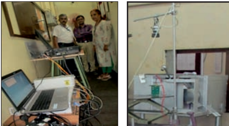
Fig. 22: Test Set up for Radiation sensor by SAC/ISRO, at BRIT-Calibration Laboratory
