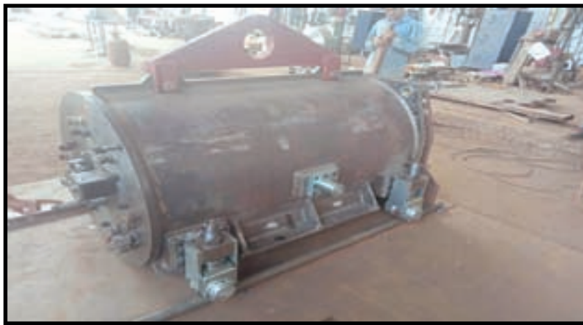
Under fabrication-New ISOMED Type Horizontal Transportation Cask (HTC) for Co-60 Source handling, transportation and storage
